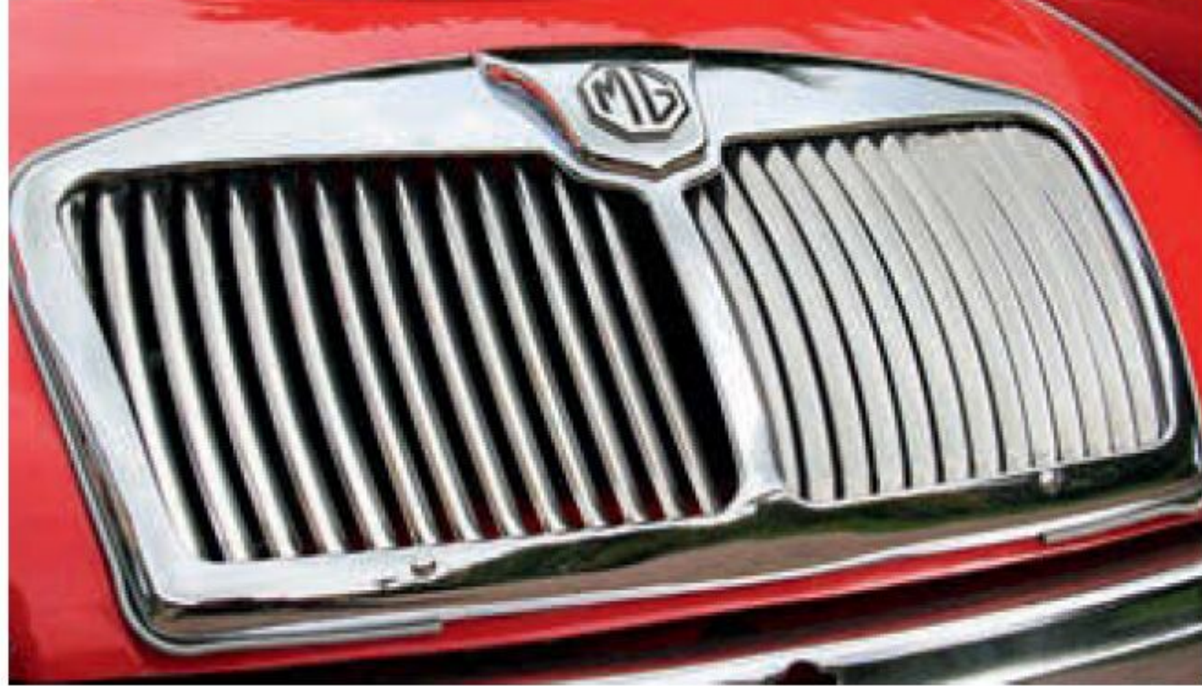
The grille of an MGA Mk1 model. Note that it sits flat to the surround.
