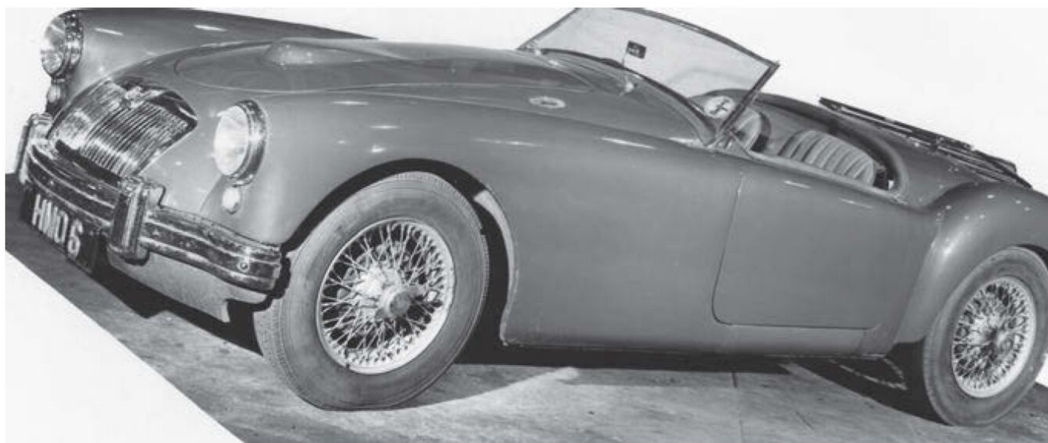
Below: Nearly there. This was the famous EX175 prototype of 1952, looking exactly as the production MGA 1500 became, but fitted with an XPAG TD engine.
